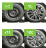
Checking if the tires are wrapped with PE film
